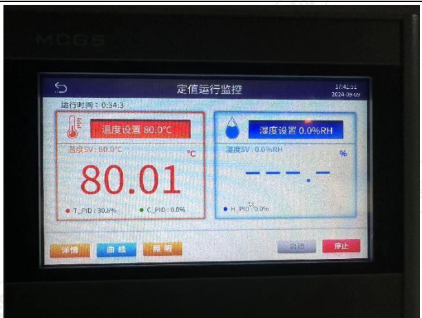
Fig.1-6 High Temperature Test Operation Interface Diagram
