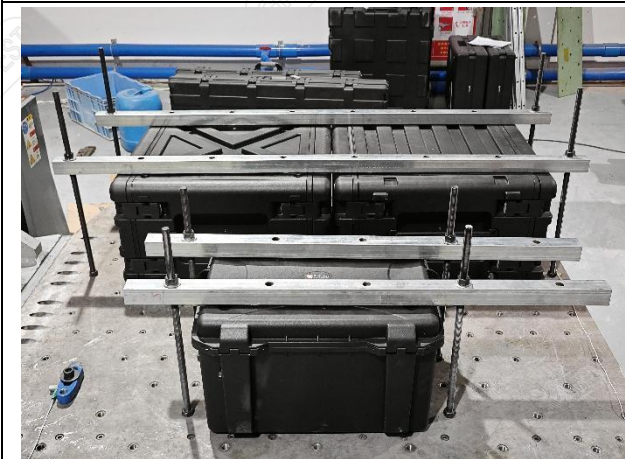
Fig.2-3 Vibration Test Subject Installation Status - X-Axis
